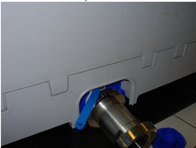
Place the key on the piston to open or close the valve. Left upper corner = CLOSED
