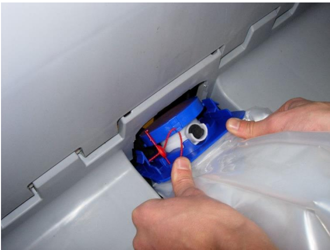
IMPORTANT, first place the underside of the clip in the channel, (inside view).
