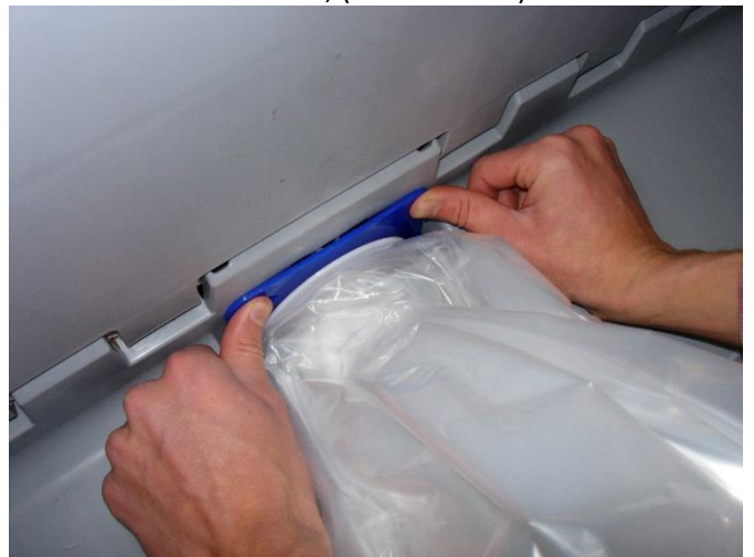
Press the top end of the clip firmly until all edges of the clip are against the container.
