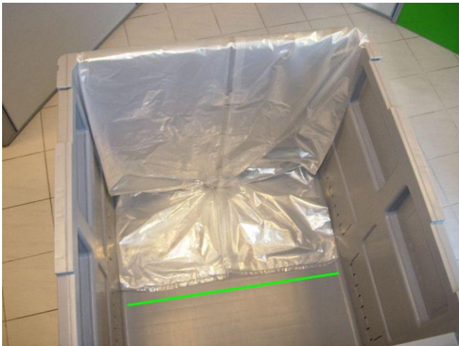
After the rear panel is in place, the bottom of the liner should still lay flat in the container.
